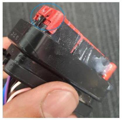
To remove the cap, pull the hook and push it away from the connector
