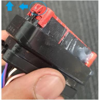
In the same time, with a small flat heat screw driver or tweezers, push the square away from the connector
