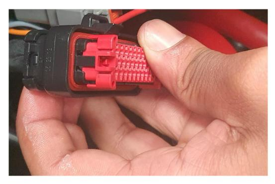
When pressing the cap back, need to feel the locker aligned with the connector and press again to fully close the connector.
